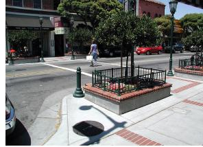
Figure 5.27: Example of a Curb Bulb-Out
