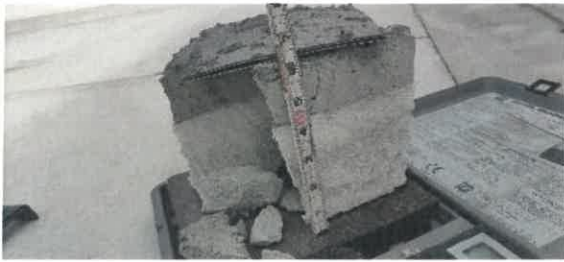
Photo #15 General overview of the make-up of core 'E'.
