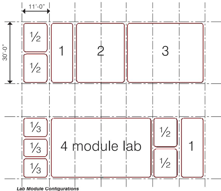
Laboratories should be organized around modular planning principles so they are constructed with standardized units or dimensions for flexibility and to enable a variety of uses. Modular planning is used as an organizational tool to allocate space within a building. The module establishes a grid by which walls and partitions are located. As modifications are required because of changes in laboratory use, instrumentation,
