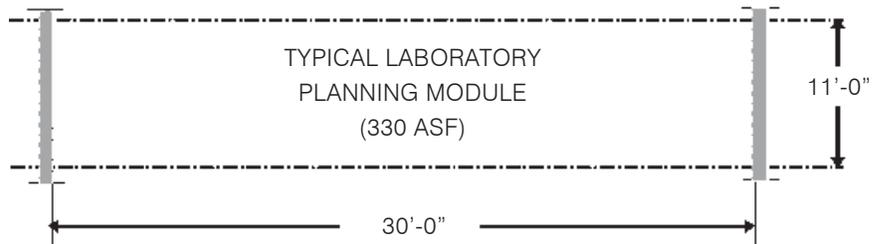
A planning module approximately 11'-0" wide by 30'-0" deep is recommended for the laboratory spaces. This module will provide adequate bench space plus space for floor standing equipment and fume hoods, and can be divided for smaller support spaces such as equipment and instrument rooms. The recommended module size will be tested against the column spacing and exterior wall locations of the proposed relocation site during the design phases, and may be adjusted accordingly.
