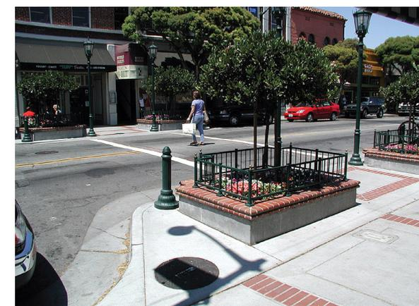
Figure 5.27: Example of a Curb Bulb-Out
